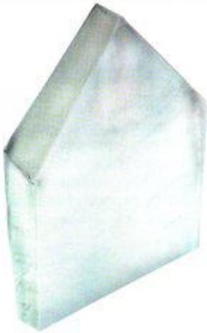
**Method's Features:** Sapphire grown by Bagdasarov method possesses high optical quality (2<sup>nd</sup> or 3<sup>rd</sup> material grade). Typical crystals grown by this method are shaped as thick rectangulars (e.g. 170mm x 200 mm x 35-38 mm). This material is ideal for manufacturing sapphire Ingots/blanks/windows of diameters 2"-8" and thickness >3 mm. Bagdasarov method is applied in manufacturing C-plane Ingots for Blue LEDs up to 8" in diameter.
